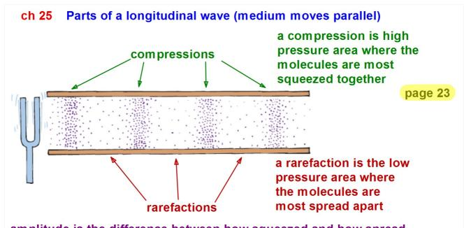
amplitude is the difference between how squeezed and how spread a longitudinal wave also has wavelength, period, and frequency
