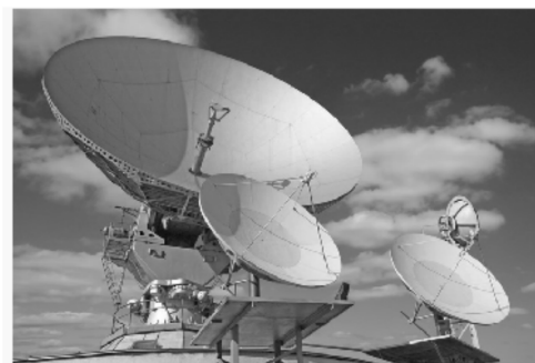
Satellite Dishes are Parabolic with the receiver at the focus.
