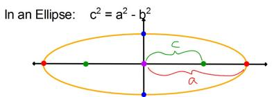
C is smaller than a because the Focus is closer to the Center than the Vertex.
