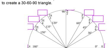
To find the coordinates of the point at 120° draw a line down to the x-axis
