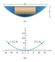
**FIGURE 1.82** (a) A parabolic satellite dish with a protective cardboard cylinder in the middle for packaging. (b) The parabola in the coordinate plane. (Example 3)
