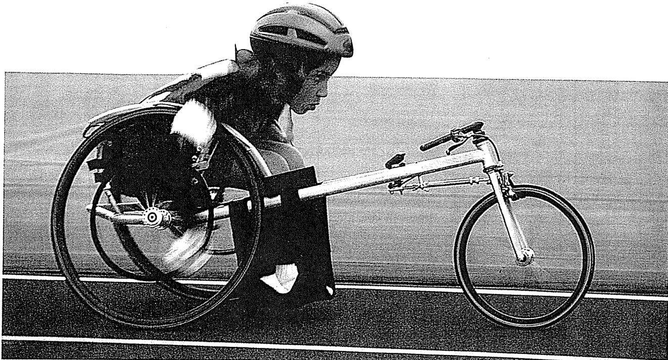
Figure 17 Wheelchairs used for racing and playing basketball often have parts made from titanium.
