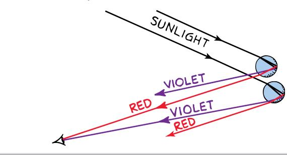
At a particular angle, you sweep out the portion of a cone, with your eye at the apex.
