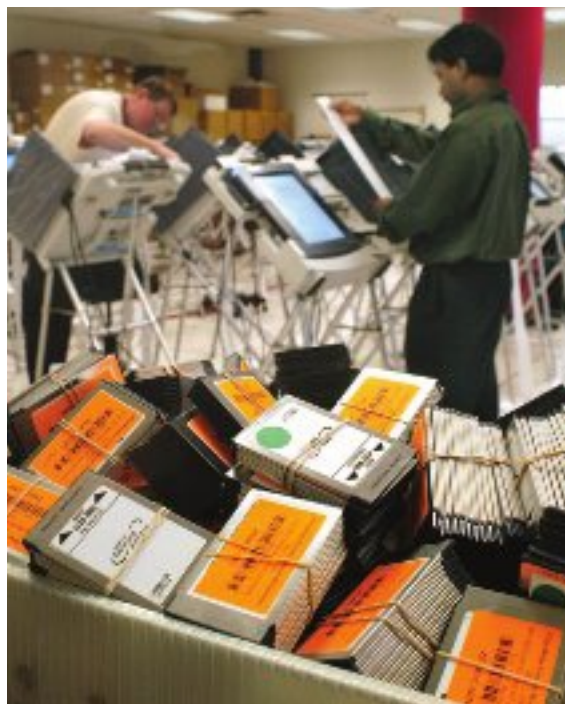
▲ Memory cards record votes cast on electronic voting machines.
