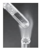
When mercury oxide is heated, it undergoes a chemical change in which it separates into the elements mercury and oxygen.
